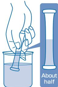
③ Immerse the aperture of the tube into the sample and release to fill the tube halfway. Invert the tube back and forth for 5-6 times.
