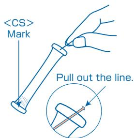
① Remove the colored line at the top of the tube to clear the aperture.
