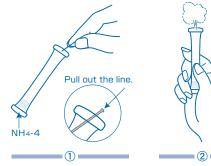
①Remove the colored line at the top of the tube to clear the aperture.
