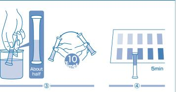
③Immerse the aperture of the tube into the sample, release the finger to fill the tube halfway. Invert the tube back and forth lightly for 10 times.
