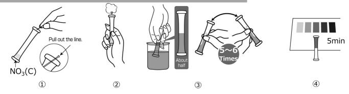
When Nitrite coexist  $\geq 1 - \langle 10mg/L \rangle$ : Remove nitrite by pretreatment agent prior to nitrate measurement. \*Nitrate cannot be measured if nitrite coexist  $\geq 10mg/L$ .
